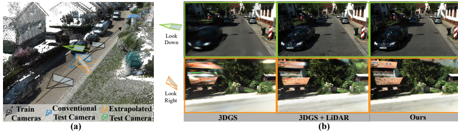
Fig. 1: (a) Illustration of Extrapolated View Synthesis (EVS) problem in urban scenes reconstructed with forward-facing cameras. In contrast to conventional test cameras similar to training camera poses, we evaluate view synthesis on cameras distant from training camera distribution. (b) Qualitative comparison on EVS to baselines.
